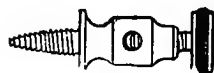
FIG. 4.—One form of binding post. The screw at its end is intended for contact with the electrical conductor, and the line wire is inserted in the hole through the centre, where it is held tight by the thumb screw.
